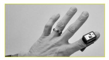
Kinesia Sensor to Measure Three-dimensional Movement
